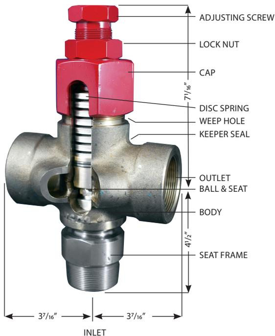
Designed for protection against over-pressure for vessels, pumps, lines, etc. It is a rugged and versatile valve capable of handling a wide range of pressures.
